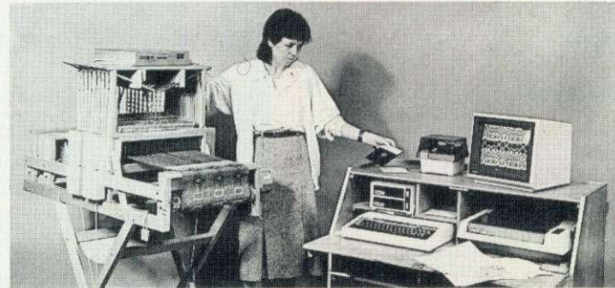
Harris Designer Loom station includes a 16 shaft 15in loom and BBC micro
